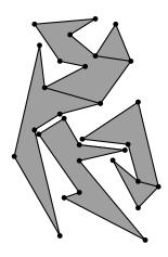
Towards an efficient algorithm Partitioning into monotone pieces Triangulating a monotone polygon Triangulating a simple polygon
