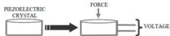
Fig 1. Principle of direct piezoelectric effect
