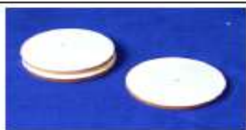
A. Normal Ultrasonic Piezoelectric Ceramic Transducer (Disc Shape)
