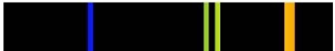
Emission line spectrum with thermal line broadening
