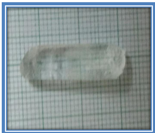
Fig. 1. Photograph of 3 wt % LC doped KDP crystal
