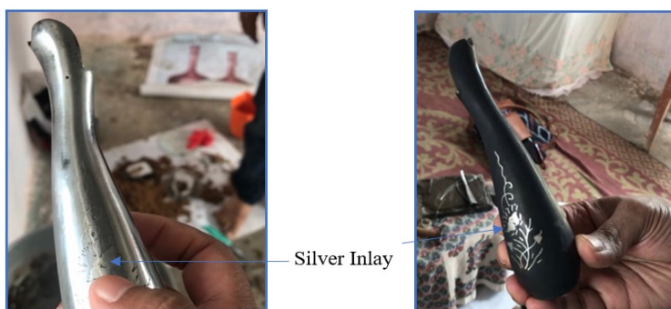
Fig. 2. Bidri zinc alloy: a) before treatment (Unpatinated surface); b) after treatment with Bidar fort clay
