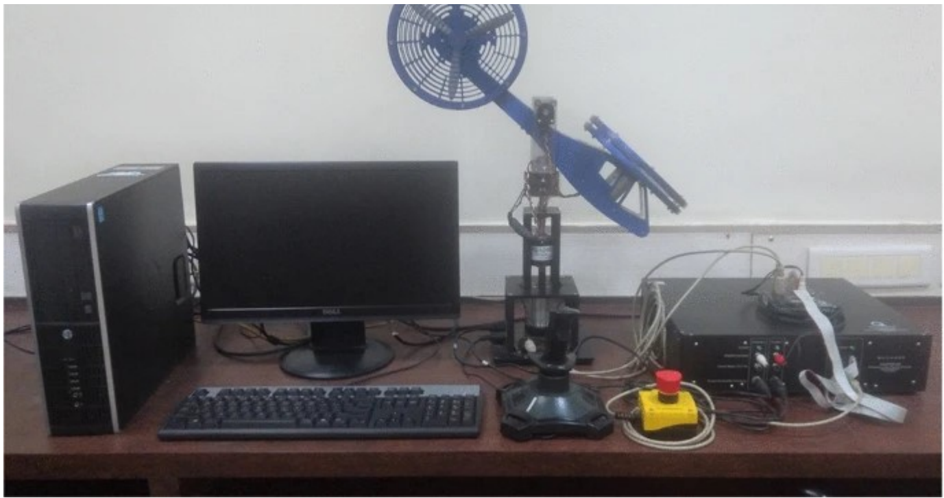
Laboratory setup of 2-DOF helicopter system
