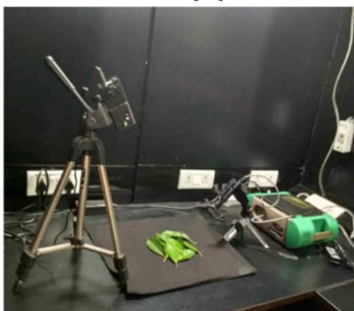
Figure 2.a :FieldSpe4 Spectroradiometer Setup for Spectral measurement Figure 2.b: Raw DN Spectral signatures of Plant samples
