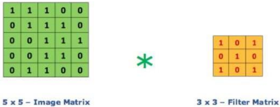
Figure 7: Image matrix multiplies kernel or filter matrix
